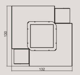
For the people who have bigger garden and love hearths we recommend our hearth. In production process we use laser cutting technology from 3mm metal sheet, forming on the edge press and connecting by bolts. Product is corrosion protected by heat resistant paint. Hearth can be used in the garden or terrace. Wood storage place helps to enjoy relax moments in your garden.
