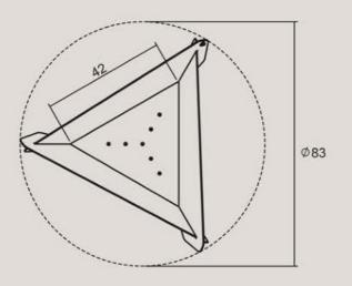
Following the customers who like mobility of the product we created small triangle hearth. Product made with 3mm metal sheet, laser cutting. Item is corrosion protected painted by heat resistant paint. Thanks to light and smart construction hearth can be folded and moved to another place. Can be used in any environment where open fire is allowed.
